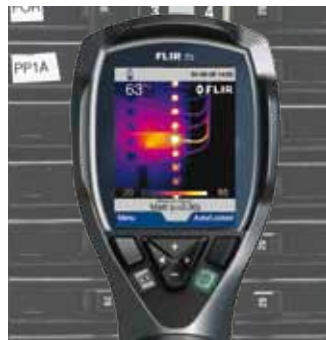
FLIR i5, temperature in 6,400 spots
