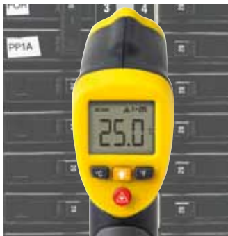
IR thermometer, temperature measurement in one spot
